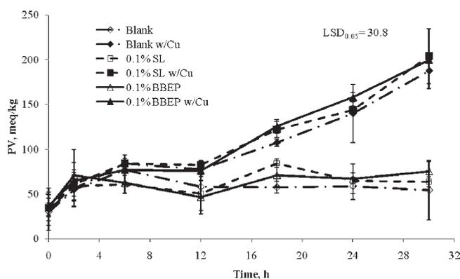
**Figure 5.** PV development of egg phospholipids in liposome at 37 °C in the presence of cumene hydroperoxide (40  $\mu$ M in liposome). Error bars represent SD from duplicate preparations. The concentration of SL and BBEP is 1000 ppm based on EPL. For treatment abbreviations, refer to the footnotes of **Tables 1** and **2**.
